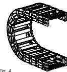
Fig. A The chain can be fixed frontally, inner or outer radius, (Fig A)
